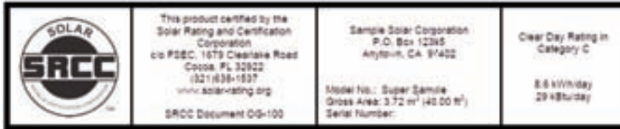
Figure 10.3. Each solar collector also will have a collector certification sticker from the OG 100 test.
