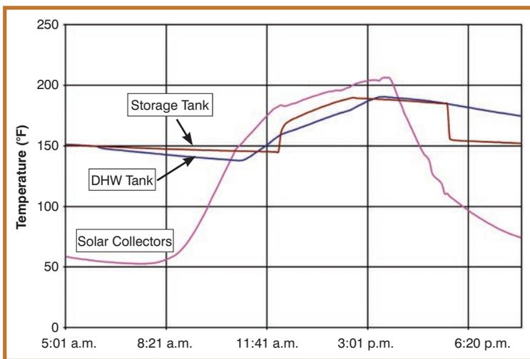
**Figure 2:** Logged data on heat storage, DHW use and night sky radiant cooling for a system in Virginia during the summer.
