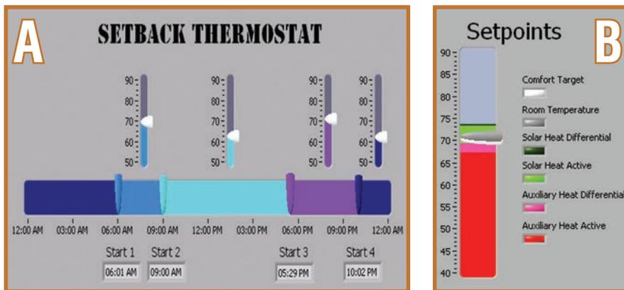
**Figure 1a (left):** User interface for controlling a setback thermostat in a non-mass heating zone. **Figure 1b (right):** Informational graphic showing the two-stage heating settings of an in-mass radiant zone.
