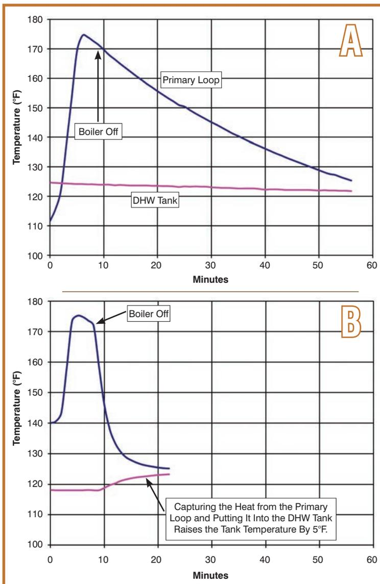
**Figure 3a (top):** With normal controls, after the boiler is turned off, the stranded heat is slowly lost to the mechanical room. **Figure 3b (bottom):** With central control and integrated logic, the system can keep pumps running to capture the stranded heat in the primary loop and move it to the DHW tank.
