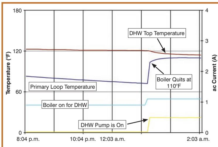
**Figure 4:** A boiler failure (safety lockout) is the cause of a lack of DHW.
