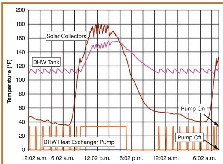
**Figure 5:** In this home, the DHW recirculator is on continuously and manages to waste all of the solar heat stored in the DHW tank within six hours after sunset.
